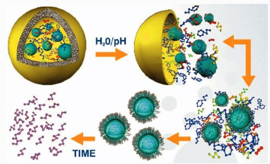
Two or more ingredients that would react with each other if put together can be separated and provided consecutively by placing one in the nanosphere and the other in the microsphere.
